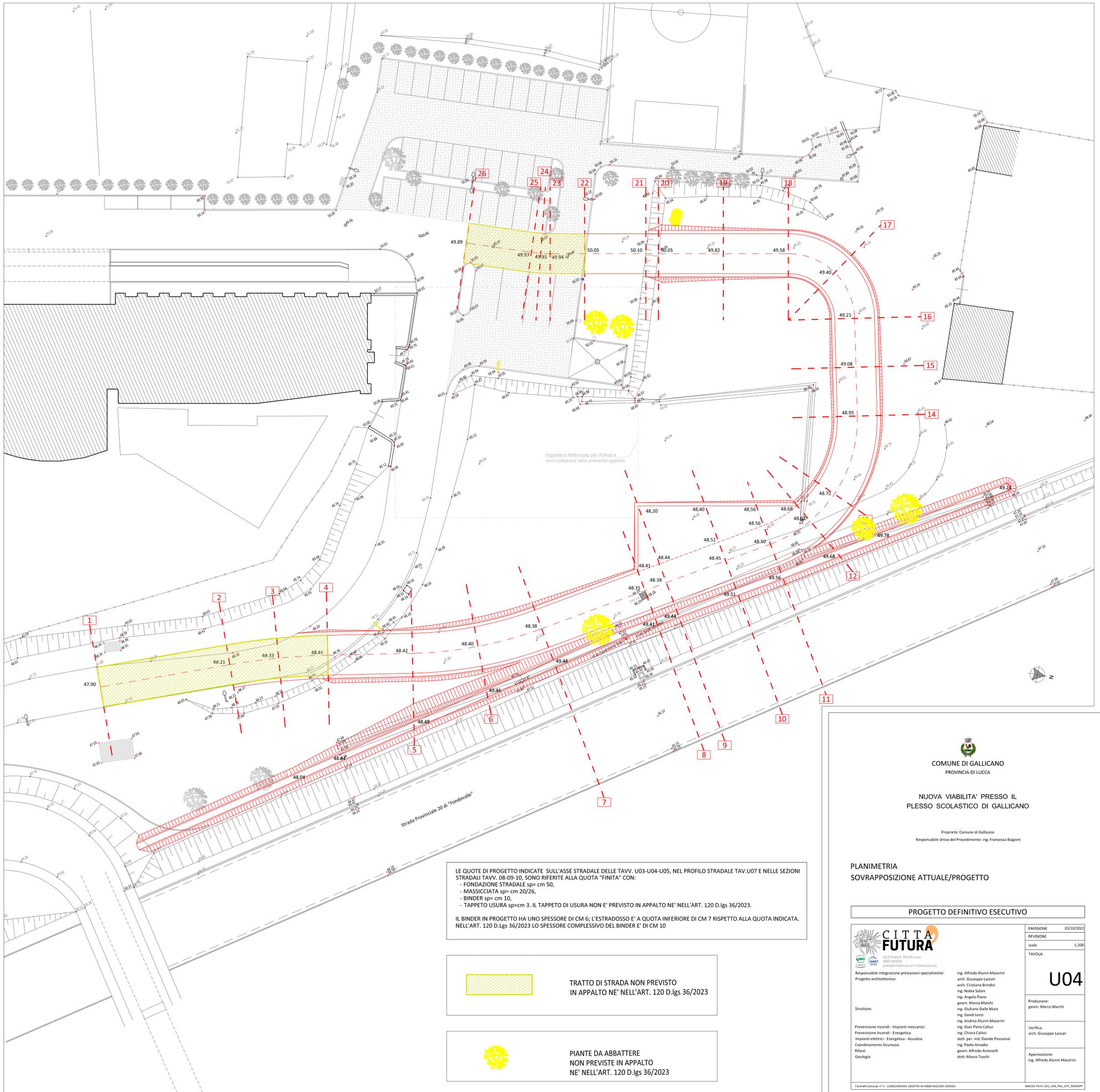
LE QUOTE DI PROGETTO INDICATE SULL'ASSE STRADALE DELLE TAVV. U03-U04-U05, NEL PROFILO STRADALE TAV.U07 E NELLE SEZIONI STRADALI TAVV. 08-09-10, SONO RIFERITE ALLA QUOTA "FINITA" CON:
